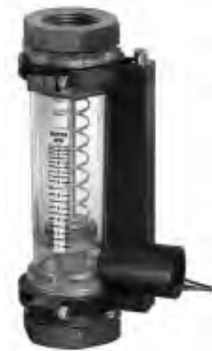
Each switch kit consists of a ring shaped ceramic magnet, that fits around the flow meter piston, and a proximity switch in a housing that clamps to the body of the flow meter. As the magnet moves with the piston, its
