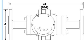
"Flow up" or "flow down" dimensions are the same. Scale numbers are turned 90° to be right reading. For additional information on flanged connection see page 129.
