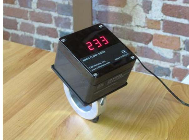
The flowmeter clamps onto a pipe, with two flow-sensing probes projecting into the pipe through 3/16-in. drilled holes. It seals directly to the pipe; no cutting or welding is required for installation. Because each flowmeter is made and calibrated for a specific size of pipe, the display indicates flow directly, with no setup or adjustment.
